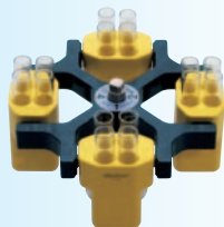
Swing-out rotor, 4-place, n= 4,000 min -1 , RCF 2,665, for max. 4 x 100 ml.
